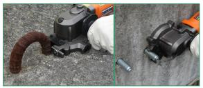
Get rid of unwanted protruding rebars or anchor bolts by cutting them cleanly at surface level.
